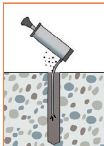
Clean hole (blowing)
