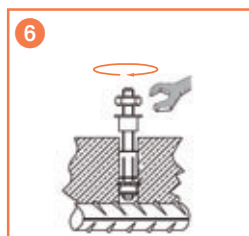
Remove the hex nut, washer and distance sleeve.
