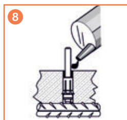
Fill annular gap completely with injection mortar.
