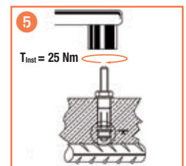
Apply recommended fastening torque with a calibrated torque wrench.
